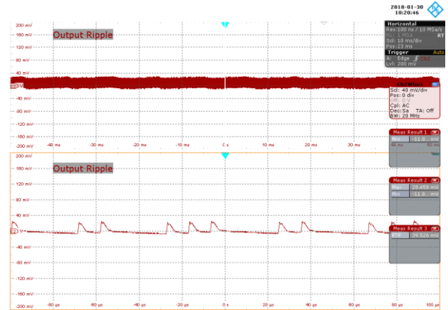
Figure 113 – 115 VAC 47 Hz, 25% Load. CH1: V_{OUT} , 40 mV / div., 10 ms / div. Zoom: 20 \mu s / div. Voltage Ripple ( V_{OUT(PK-PK)} ) = 39.5 mV).
