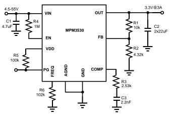
Figure 3: 3.3V Output Typical Application Circuit
