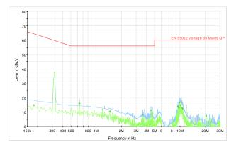
Radiated Emission, EN55022 Class B Vout=3.3V Input Pi Filter: 10uF, 4.7uH, 10uF
