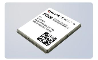
BG96 is a series of LTE Cat M1 and Cat NB1 module offering a maximum data rate of 375kbps downlink and uplink. It features ultra-low power consumption, and provides pin-to-pin compatibility with Quectel LTE module EG91, Cat NB1 (NB-IoT) module BC95, UMTS/HSPA modules UG95/UG96 and GSM/GPRS module M95.
