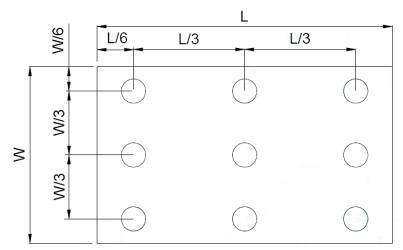
Bmax : The measured maximum luminance of all measurement position. Bmin : The measured minimum luminance of all measurement position.
