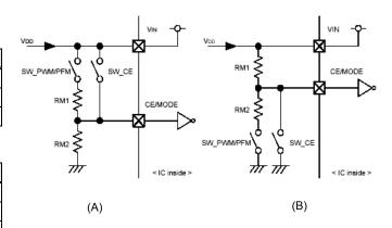
Intermediate voltage can be generated by RM1 and RM2. Please set the value of each R1, R2, RM1, RM2 from few hundreds  $k\Omega$  to few hundreds  $M\Omega$ . For switches, CPU open-drain I/O port and transistor can be used.
