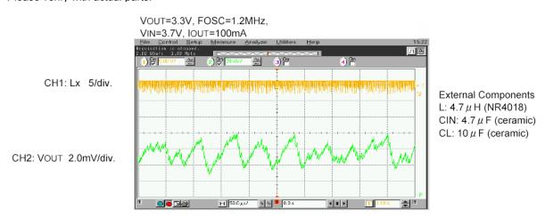
18. Please note the inductance value of the coil. The IC may enter unstable operation if the combination of ambient temperature, setting voltage, oscillation frequency, and L value are not adequate.
