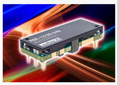
▶ The fully isolated RBE-12/20-D48 series accepts a 36 to 75 Volt DC input voltage range (48 VDC nominal) and converts it to a fixed 12Vdc output. Wideband output ripple and noise is a low 100mV (typical), peak-to-peak. The RBE is supplied in a low-profile DOSA standard eighth-brick package measuring 58.4 x 22.9 x 10.2 mm (2.3 x 0.9 x 0.4 inches).
