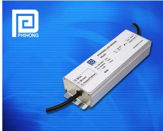
The 125W driver series is rated for universal inputs of 100 to 304VAC, which is ideal for both North American 120 or 277VAC and European 230 to 240VAC mains voltage ranges. The lighting power supplies are water resistant and fully potted, featuring the ingress protection rating IP65. The series also features an extremely wide range of operating temperatures, from -40°C to +60°C, making it ideal for a variety of applications outside of climate-controlled environments.
