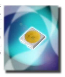
Due to its enhanced resin mixture for encapsulation an excellent lifetime up to 50k hours is reached. The package has an outline of 3.5 (L)  $\times 3.5$ (W)  $\times 1.1$ (H) mm and is therefore slightly different from other DomiLED packages. It features besides an electrically isolated heat sink for optimal heat dissipation a large light emitting surface with a diameter of 3 mm.
