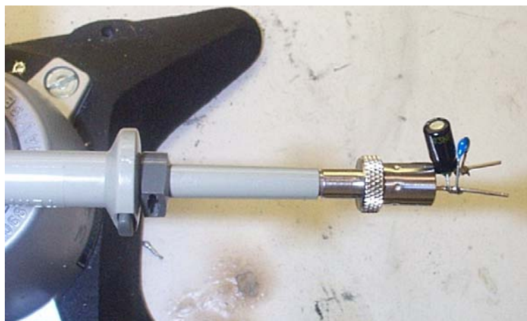
Figure 28 – Oscilloscope Probe with Probe Master 4987BA BNC Adapter (Modified with Wires for Probe Ground for Ripple measurement and Two Parallel Decoupling Capacitors Added).
