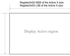
Register0x04 MSB of the Active Y size Register0x05 LSB of the Active Y size
