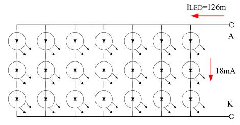
The constant current source is needed for white LED back-light driving.
