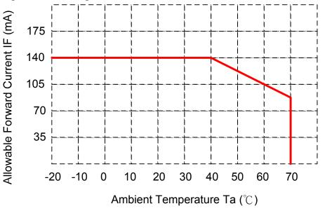
Note7 : This is panel surface temperature, not ambient temperature. Note8 : When LCM be operated over than 40°C , the life time of the LED back-light will be reduced.
