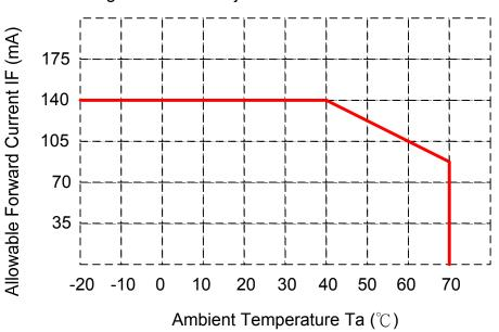
back-light should be adjusted to 105mA max
