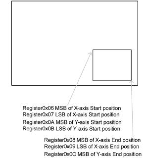
Register0x0D LSB of Y-axis End position
