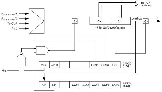
**Table 52.** CMOD Register CMOD - PCA Counter Mode Register (D9h)
