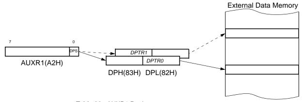
**Table 30.** AUXR1 Register AUXR1- Auxiliary Register 1(0A2h)
