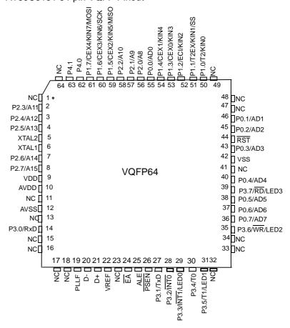
Figure 2. AT89C5131 64-pin VQFP Pinout
