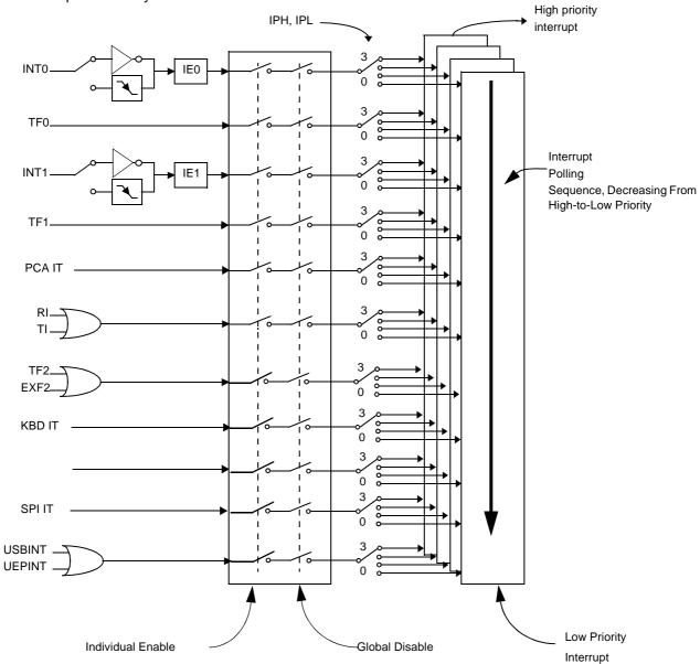
Each of the interrupt sources can be individually enabled or disabled by setting or clearing a bit in the Interrupt Enable register (Table 65). This register also contains a global disable bit, which must be cleared to disable all interrupts at once.
