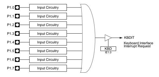
Figure 41. Keyboard Input Circuitry
