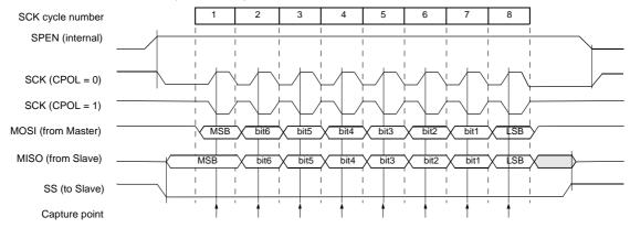
Figure 46. Data Transmission Format (CPHA = 1)
