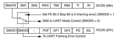
When this feature is enabled, the receiver checks each incoming data frame for a valid stop bit. An invalid stop bit may result from noise on the serial lines or from simultaneous transmission by two CPUs. If a valid stop bit is not found, the Framing Error bit (FE) in SCON register (See Table 60) bit is set.
