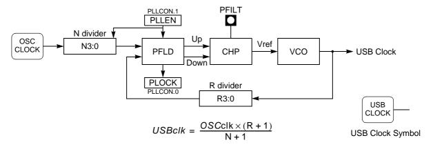
Figure 8. PLL Filter Connection
