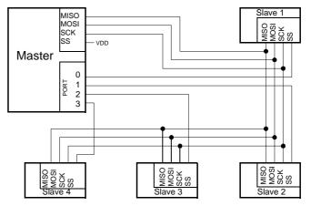
The Master device selects the individual Slave devices by using four pins of a parallel port to control the four SS pins of the Slave devices.
