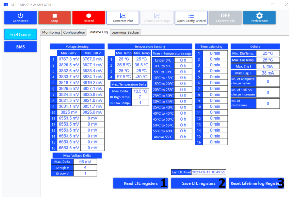
Figure 67: Lifetime Log View
