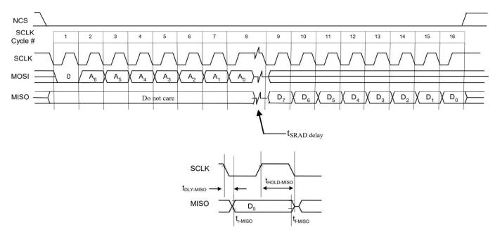
NOTE: The 0.5/fSCLK minimum high state of SCLK is also the minimum MISO data hold time of the PAW-A350. Since the falling edge of SCLK is actually the start of the next read or write command, the PAW-A350 will hold the state of data on MISO until the falling edge of SCLK.
