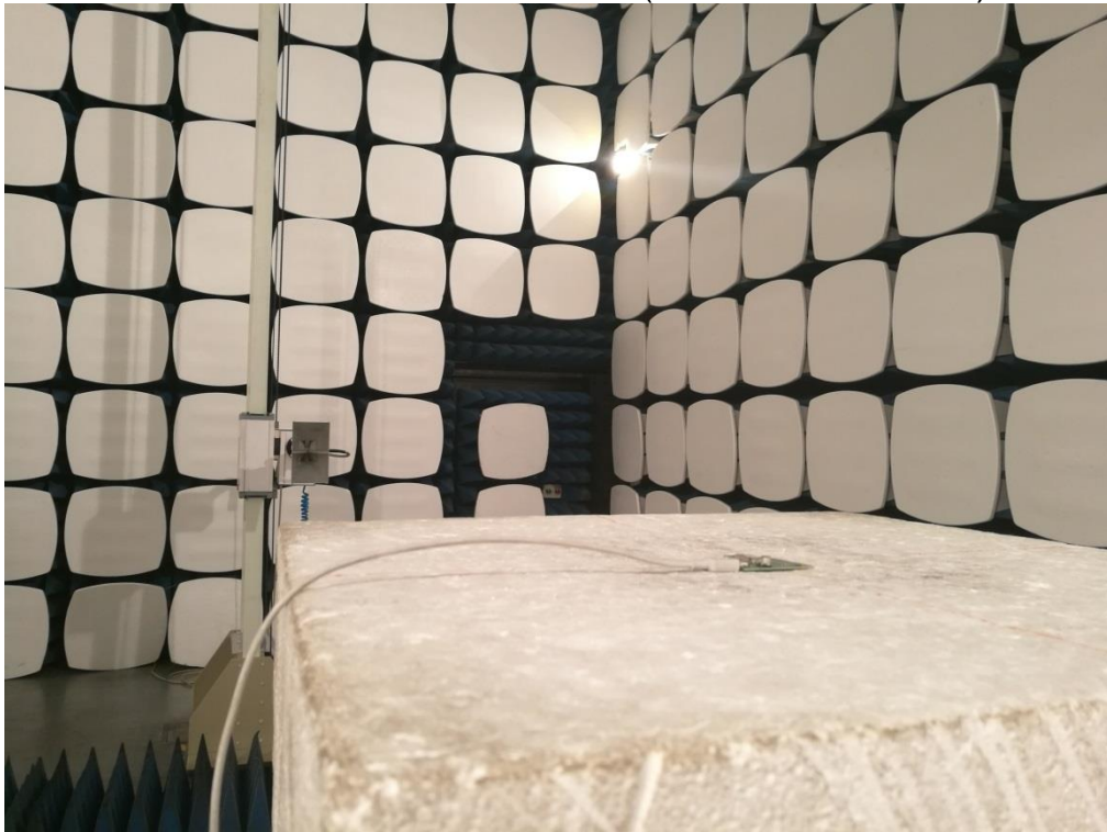
Radiated Emission Above 1GHz (for Ceramic Antenna)
