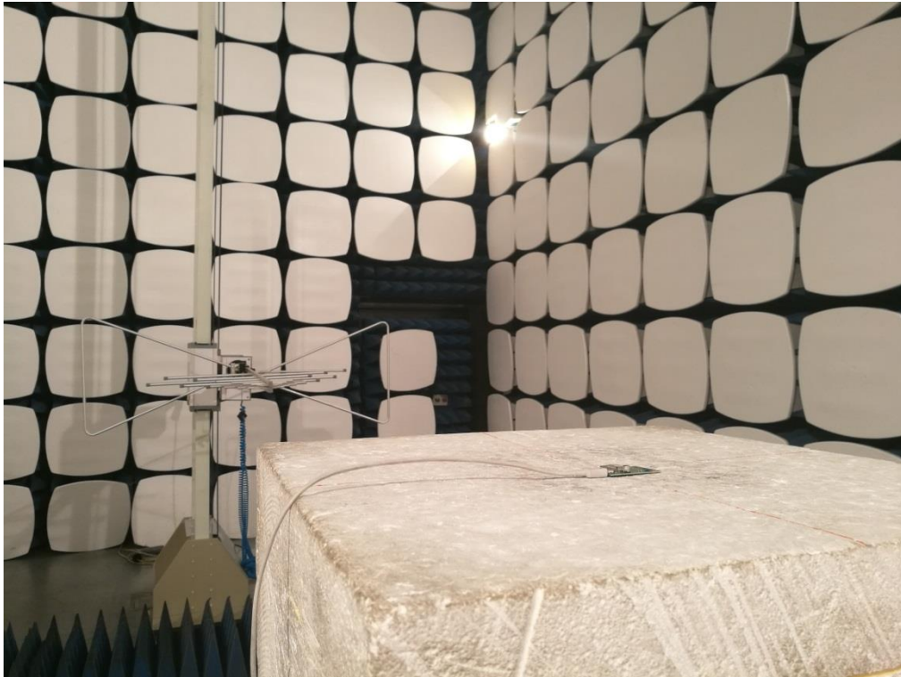
Radiated Emission Below 1GHz (for Ceramic Antenna)
