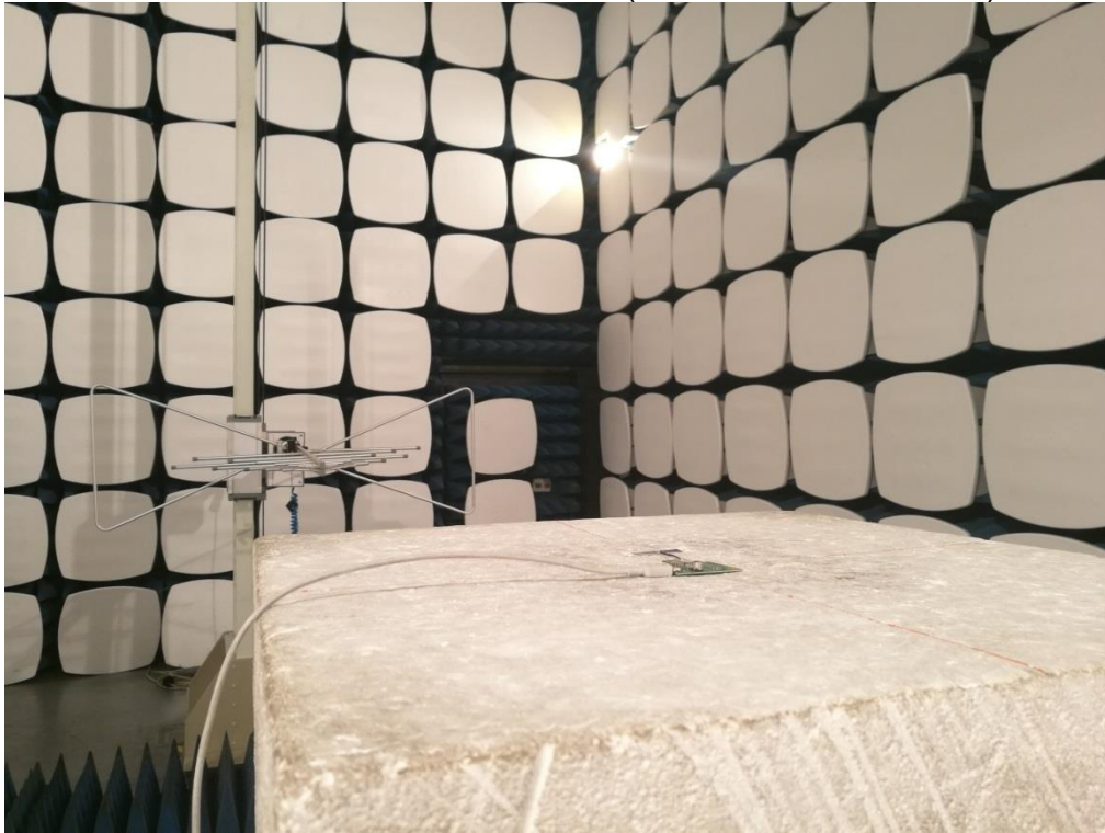
Radiated Emission Below 1GHz (for External antenna B)
