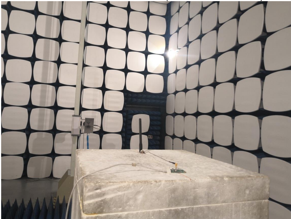
Radiated Emission Above 1GHz (for External antenna A)
