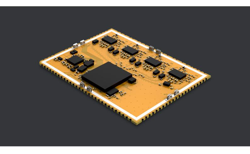
Pineapple is an 802.11ax Wi-Fi 6 and Wi-Fi 6E radio module for ultra-high speed enterprise connectivity. It is based on Qualcomm QCN9074 chipset for 2.4/5/6 GHz IEEE802.11ax/ac/n/g/b/ax applications. New radio can perform access point and station functionality with 4x4 MIMO (4 spatial streams). Pineapple is a wireless LAN radio with native 160 MHz support.
