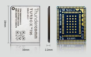
The TurboX T95 SOM (System On Module) is based on new generation of LTE Modem and purpose-built for the low power wide area Internet of Things (IoT) applications. It integrates all key innovations required to build cellular-enabled IoT products and services into a single module, including 3GPP Rel. 14 compliant LTE Cat M1/Cat NB2, E-GPRS connectivity, an ARM Cortex A7 application processor, integrated GNSS, hardware-based security, capable of cloud services, and rich set of development tools.
