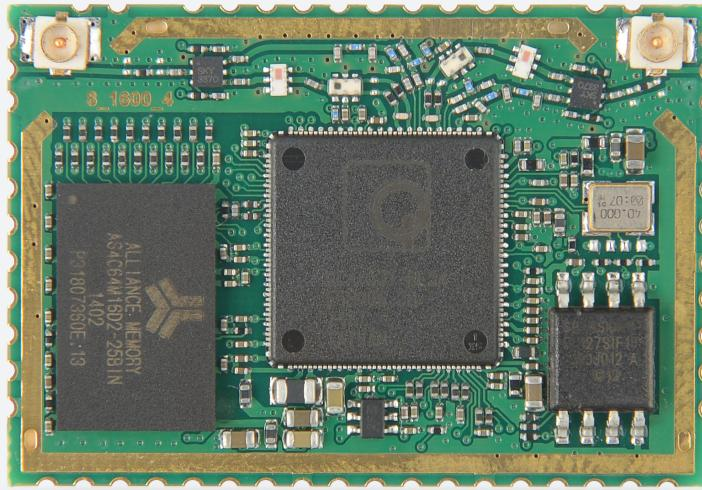
Lima has 802.11N 2x2 radio supporting up to 300 Mbps data-rate and comes in two versions: commercial or industrial temperature
