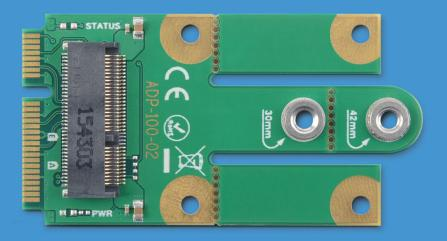
It is an adapter for BLACK bean and other M.2 form factor radio modules that fit into the standard mini PCI express slot. The adapter supports PCIe and USB2.0 system bus interfaces. It also allows connecting mini PCI express modules such as LTE, 3G, GPS, and Bluetooth. No drivers are necessary for this M.2 to mini PCI express card adapter.
