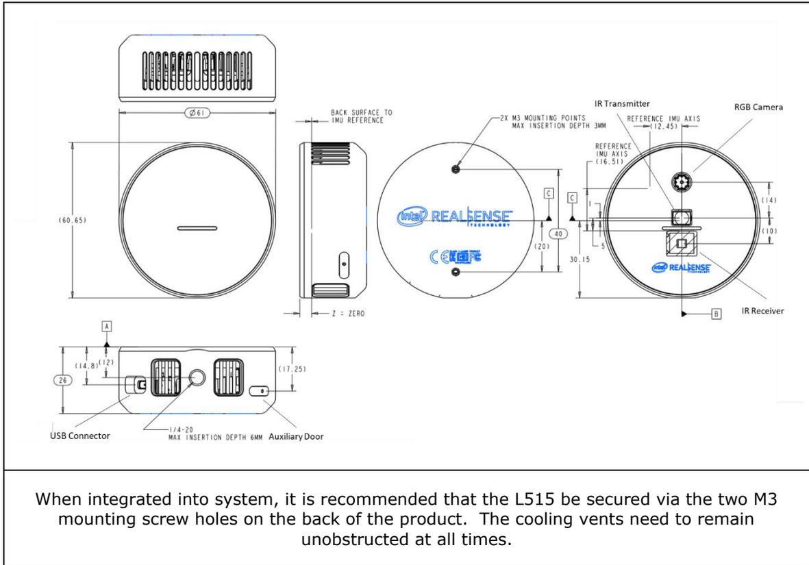
Figure 6-2. Intel® RealSense™ LiDAR Camera L515 Cooling Vents
