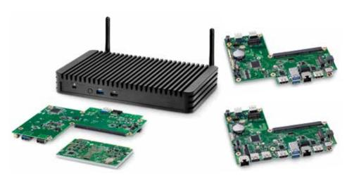
Available with two carrier board and chassis options: expandable and dual LAN.
