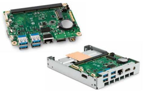
Available as a carrier board only option or with a thermal solution.
