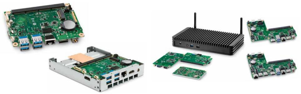
Available as a carrier board only option or with a thermal solution.
