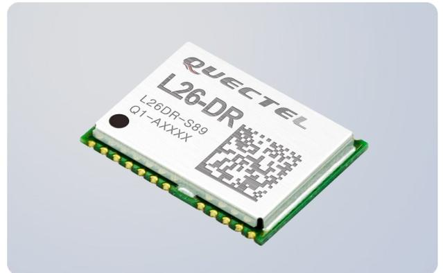
L26-DR is a concurrent multi-GNSS receiver module with dead reckoning solution. It is equipped with 6-axis sensor MEMs and a powerful GNSS core. The module provides high sensitivity, fast GNSS signal acquisition and tracking with low system integration effort.
