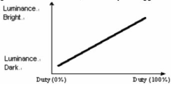
2. ADJ signal =  $0 \sim 5.0V$ , operation frequency :  $300Hz\sim1KHz$
