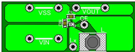
For the  $V_{IN}$ ,  $V_{OUT}$ ,  $V_{SS}$ ,  $CE$ , please put the wire.
