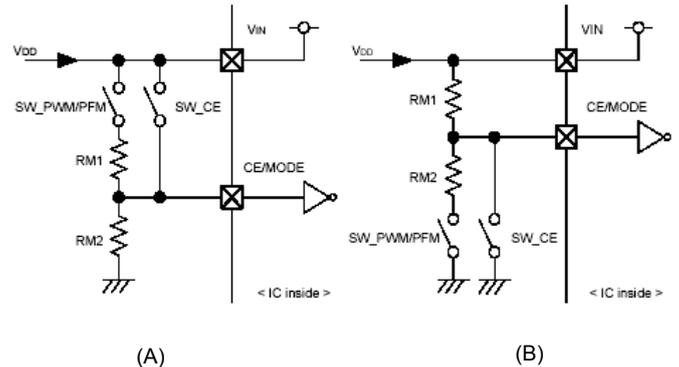
Intermediate voltage can be generated by RM1 and RM2. Please set the value of each R1, R2, RM1, RM2 from few hundreds  $k\Omega$  to few hundreds  $M\Omega$ . For switches, CPU open-drain I/O port and transistor can be used.
