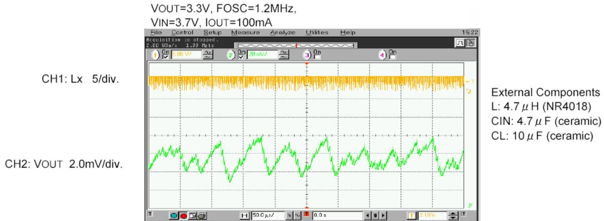
18. Please note the inductance value of the coil. The IC may enter unstable operation if the combination of ambient temperature, setting voltage, oscillation frequency, and L value are not adequate. In the operation range close to the maximum duty cycle, The IC may happen to enter unstable output voltage operation even if using the L values listed below.
