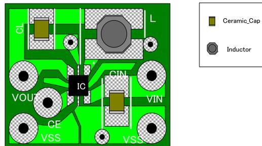
For the  $V_{IN}$ ,  $V_{OUT}$ ,  $V_{SS}$ ,  $CE$ , please put the wire.
