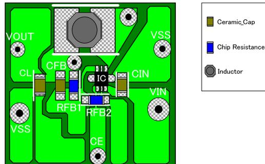
For the  $V_{IN}$ ,  $V_{OUT}$ ,  $V_{SS}$ ,  $CE$ , please put the wire.
