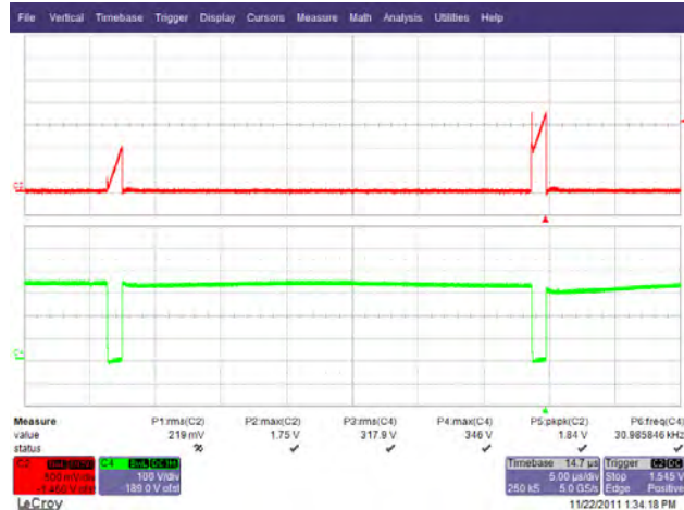
Figure 46 – 265 VAC, 50 Hz Output Short Condition. Upper: I_{DRAIN} , 500 mA / div. Lower: V_{DRAIN} , 100 V, 5μs / div.
