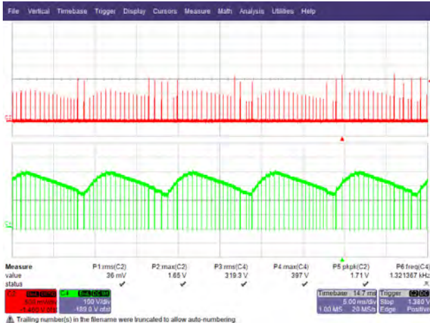
Figure 45 – 265 VAC, 50 Hz Output Short Condition. Upper: I_{DRAIN} , 500 mA / div. Lower: V_{DRAIN} , 100 V, 5ms / div.
