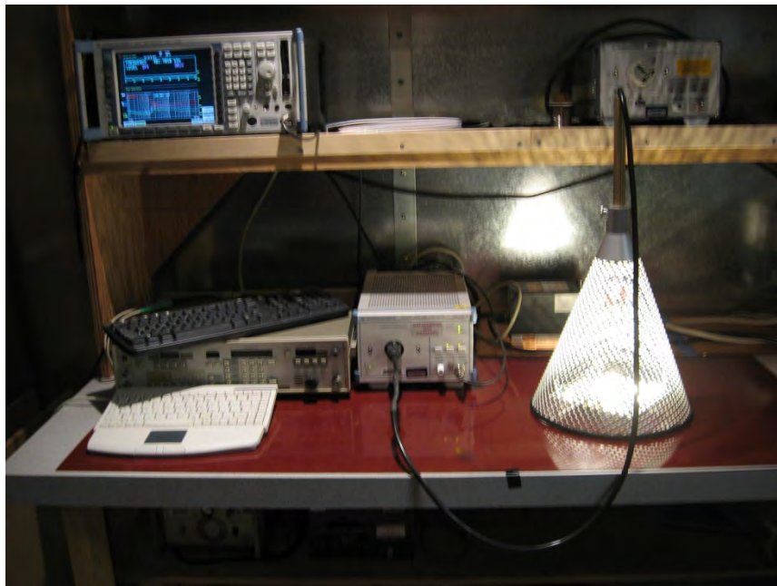
Figure 53 – EMI Test Set-up With the Unit and LED Load Placed Inside the Cone.
