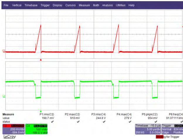
Figure 38 – 185 VAC, 50 Hz. Upper: I_{DRAIN} , 200 mA / div. Lower: V_{DRAIN} , 100 V, 5 ms / div.
