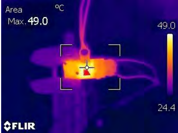
Figure 17 – Top Side. U1- LNK460VG: 49 °C.
