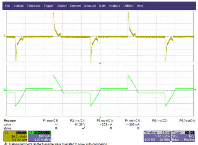
Figure 60 – 45° Conduction Angle. Upper: I_{IN} , 50 mA / div. Lower: V_{IN} , 100 V, 5 ms / div.
