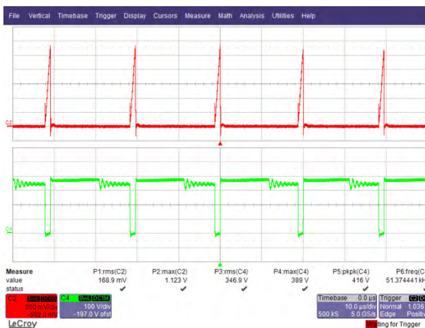
Figure 48 – 265 VAC, 50 Hz. Upper: I_{DRAIN} , 0.1 A / div. Lower: V_{DRAIN} , 100 V / div., 10 \mu s / div.
