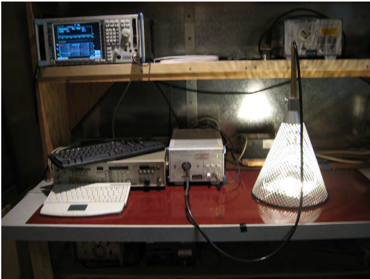
Figure 81 – EMI Test Set-up with the Unit and LED Load Placed Inside the Cone.
