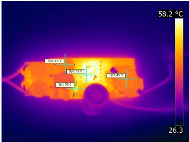
Figure 23 – Top Side. U1- LNK460VG: 58 °C.
