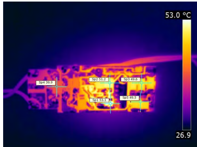
Figure 26 – Bottom Side. R4- Current Sense Resistor: 53.1 °C.
