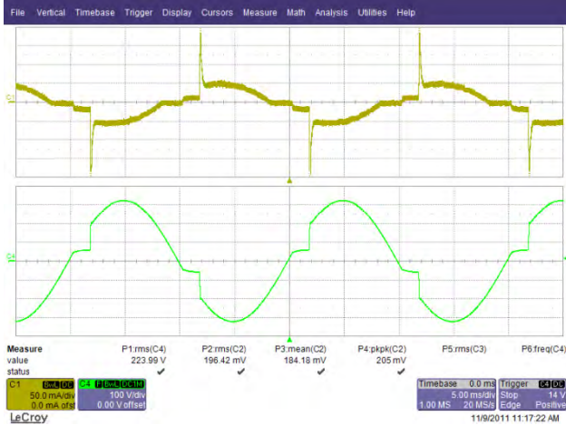
Figure 65 – 146° Conduction Angle. Upper: I_{IN} , 50 mA / div. Lower: V_{IN} , 100 V, 5 ms / div.
