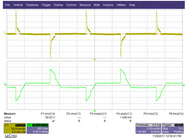
Figure 76 – 45° Conduction Angle. Upper: I_{IN} , 50 mA / div. Lower: V_{IN} , 100 V, 5 ms / div.
