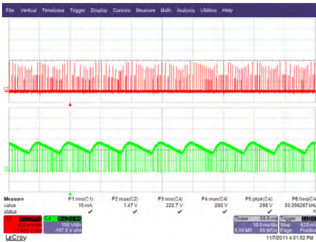
Figure 51 – 185 VAC, 50 Hz Output Short Condition. Upper: I_{DRAIN} , 500 mA / div. Lower: V_{DRAIN} , 100 V, 10 ms / div.
