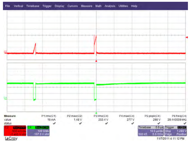
Figure 52 – 185 VAC, 50 Hz Output Short Condition. Upper: I_{DRAIN} , 500 mA / div. Lower: V_{DRAIN} , 100 V, 10 \mu s / div.
