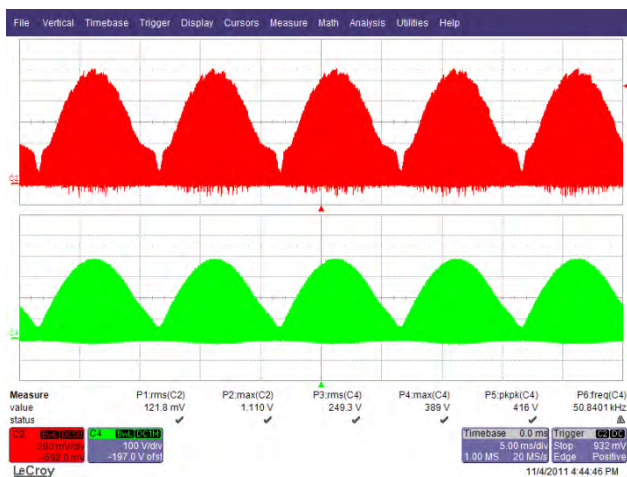
Figure 47 – 265 VAC, 50 Hz. Upper: I_{DRAIN} , 0.1 A / div. Lower: V_{DRAIN} , 100 V, 5 ms / div.
