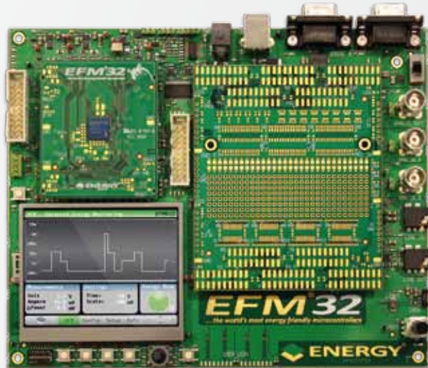
EFM32 Gecko Development Kit with MCU plug-in and prototype boards and Advanced Energy Monitoring
