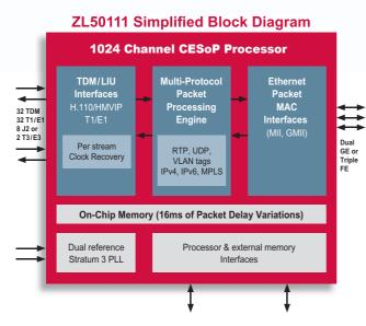
The ZL<sup>TM</sup> 50110/1/4 are Zarlink's second generation of TDM-to-Packet processors. Designed specifically for T1/E1 voice and data services emulation over packet switched networks, they optimize performance and cost efficiency of metro Ethernet applications.
