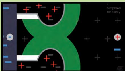
Figure 3: Reverse bias. Depletion regions overlap.
