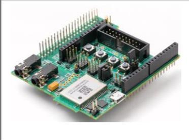
The DHAN-T-DEV incorporates a DHAN-T module loaded with DECT-ULE Device (Portable Part) communication stack as well as a thin application layer demonstrating a variety of IoT sensors and Voice capable units. This platform serves as a development tool for customizing the host application SW for a ULE Device – in particular, battery powered devices with long lifetime
