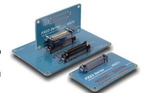
High speed transmission of up to 6 Gbps (max) is supported by the innovative contact design to ensure impedance matching. The ground contacts are situated between the adjacent differential pair contacts to reduce crosstalk for better performance.
