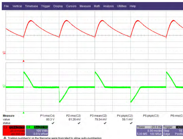
Figure 68 – 49° Conduction Angle. Upper: I_{OUT} , 20 mA / div. Lower: V_{IN} , 100 V, 5 ms / div.
