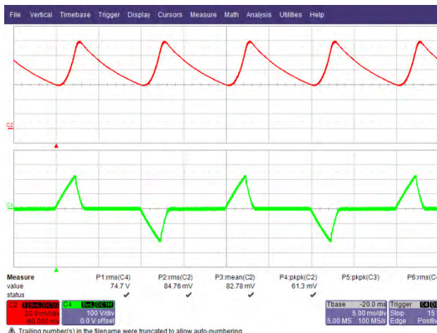
Figure 76 – 42° Conduction Angle. Upper: I_{OUT} , 20 mA / div. Lower: V_{IN} , 100 V, 5 ms / div.
