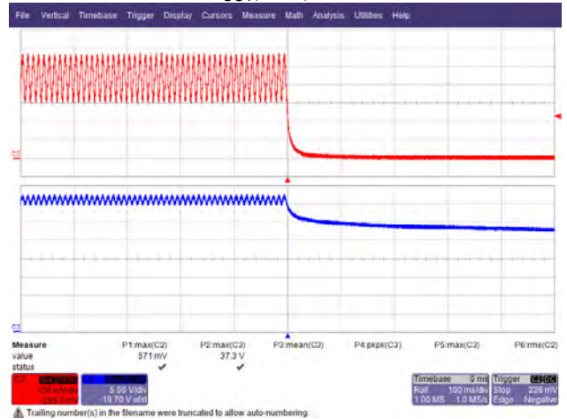
Figure 42 – 265 VAC Output Fall. Upper: I_{OUT} , 100 mA / div. Lower: V_{OUT} , 5 V, 100 ms / div.
