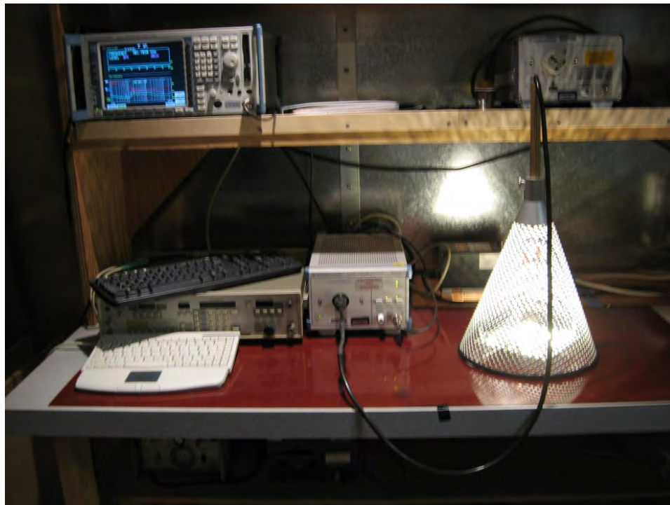
Figure 77 – EMI Test Set-up with the Unit and LED Load Placed Inside the Cone.
