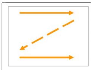
Fig. 1 Normal scan (Pin4, DPS = Low or NC)
