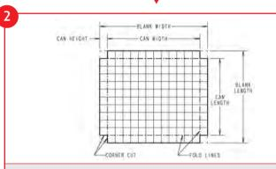
Use this diagram as a guide when cutting your etched Shield Can Sheets.
